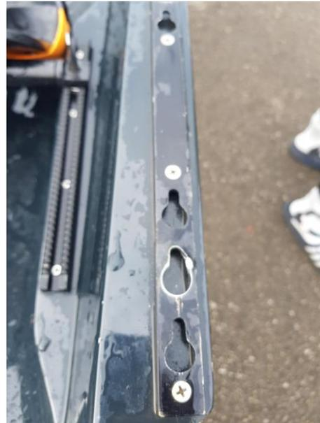
It would appear that this was a wing rigger and that the fixings may have been overtightened. There is information on the correct fitting of wing riggers [here](#) .
