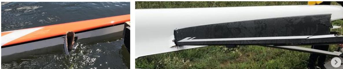
In both cases the bow, and bow ball, of one boat penetrated the hull of the other.
