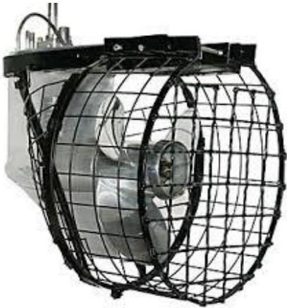
The other type forms a cylindrical cover for the propeller blade tips such that the propeller will act as a ducted fan, it looks like this:-
